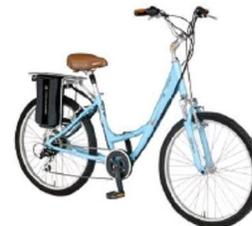
Another popular model is the electric bicycle **iZip HG1000** with a motor-scooter step through frame and 22" tires. This bicycle uses "Twist and Go" full-electric
